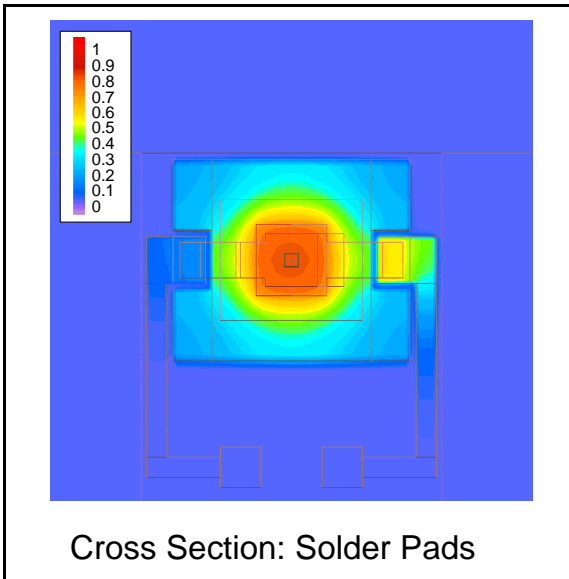
Figure 10: FPC on aluminium with standard adhesive
