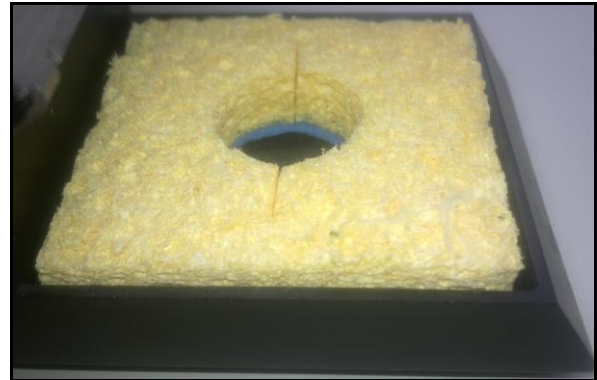
Figure 3: Example of moist sponge for cleaning soldering tips
