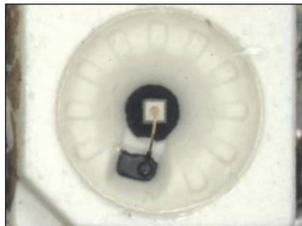
Figure 3: View of a SMT LED with blackish leadframe pads
