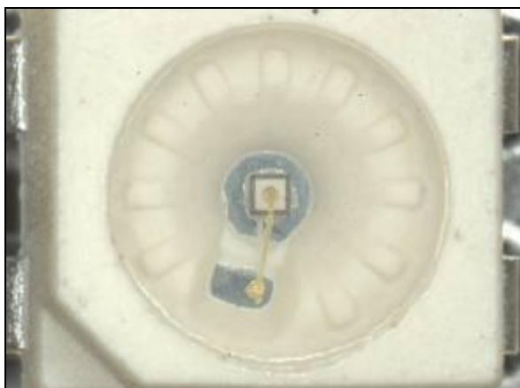
Figure 2: Picture of a SMT LED with silicone resin
