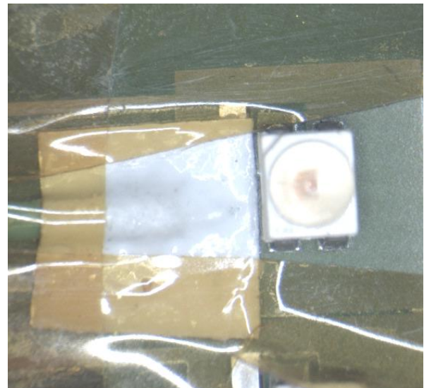
Figure 6: Example of temperature measurement on the solder pad of an LED, attachment with aluminum and polyimide tape
