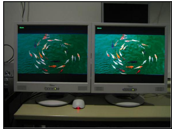
Figure 6: Display with conventional backlighting (left) and with LED backlighting (right) – the strengths lie in the red and green areas
