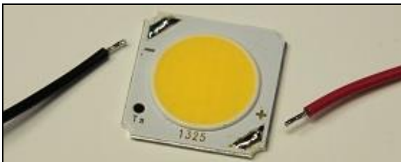
Figure 10: Pre-tinned solder pads and wires
