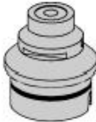
Figure 10: Sample for a Pick & Place nozzle for Golden DRAGON ARGUS LED
