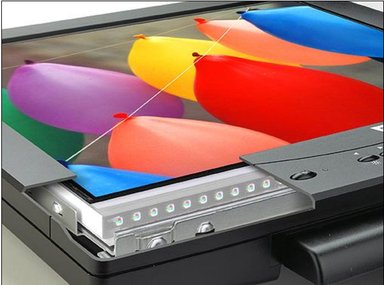
Figure 20: 17" TFT-LCD with RGB backlighting
