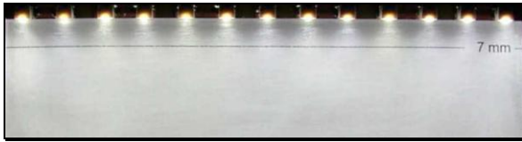
Figure 11: Compensation area for multi-color and white LEDs (LED spacing 10 mm)
